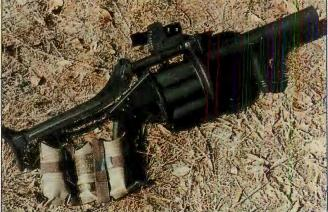
Although providing a higher rate of fire than the M79, M203 or HK69A1 single-shot 40x46mmSR grenade launchers, the MGL Mark I is heavier (11.7 pounds) and somewhat more bulky.
